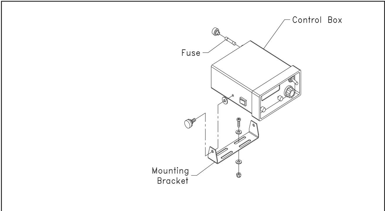
**Figure 1 - Control Box Installation**
