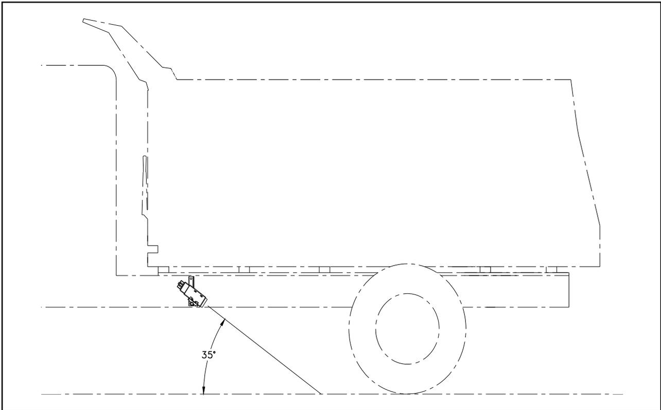
**Figure 2 - Radar Mounting Angle**
