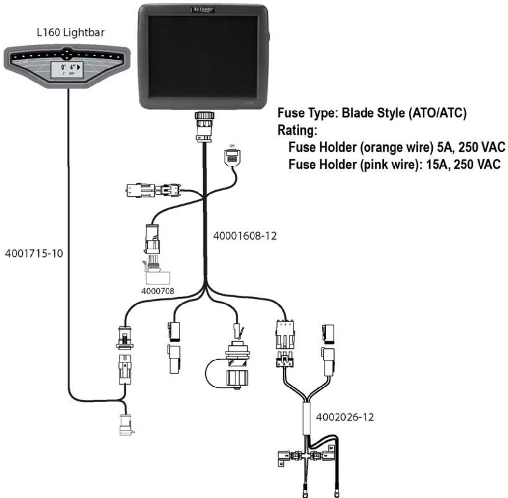
*CAUTION: The fuse is to be placed in the fuseholder in-line with the battery power cable and used with display only.*
