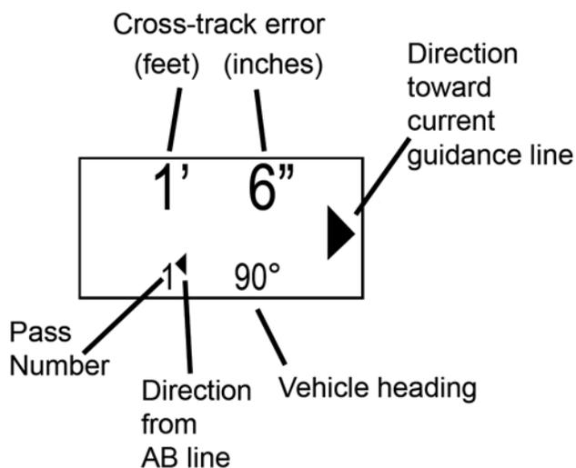
Once you have created the pattern in the display, the LCD screen will show a set of numbers and arrows. The information on this screen includes the cross-track error, direction toward the current guidance line, pass number, direction from the original AB line, and degree heading. The cross-track error is shown in feet and inches for operators using Imperial units, and centimeters for those using metric units.
