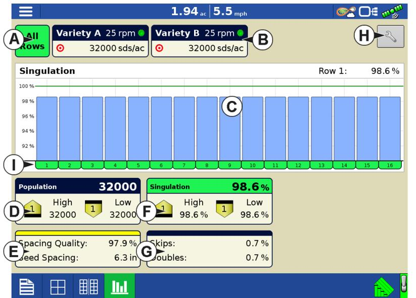
Advanced Seed Monitoring provides planter performance monitoring of seed meter singulation, skips/doubles and spacing quality, along with population and spacing information for all rows when planting compatible crops.
