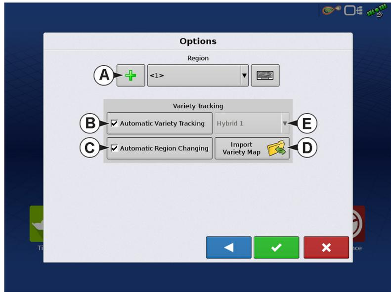
The illustration shows how the display could track two different varieties. In this example, when the harvester reaches the end of Variety 1, and moves to Variety 2, a message appears that either a new variety has been detected and the operator is notified to change regions (Automatic Variety Tracking,) or that a variety has been detected and the display is automatically changing regions. (Automatic Region Changing).
