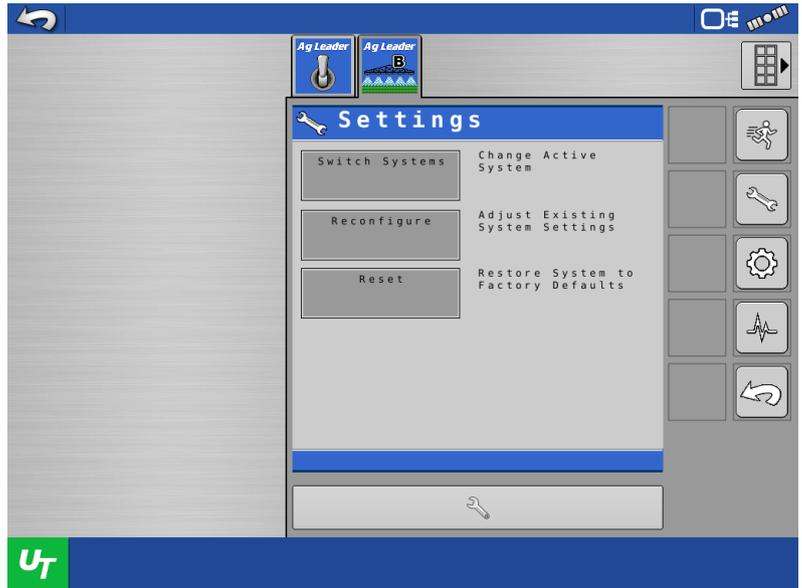
The module must reboot to switch systems. To cancel switching systems, press
