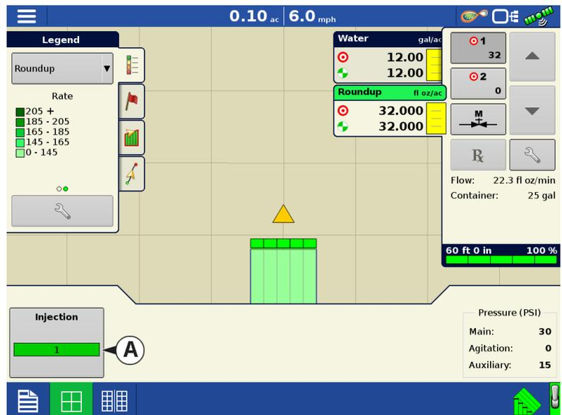
2. **Press the Prime button**—At the Injection Controls screen, press the Prime button.
