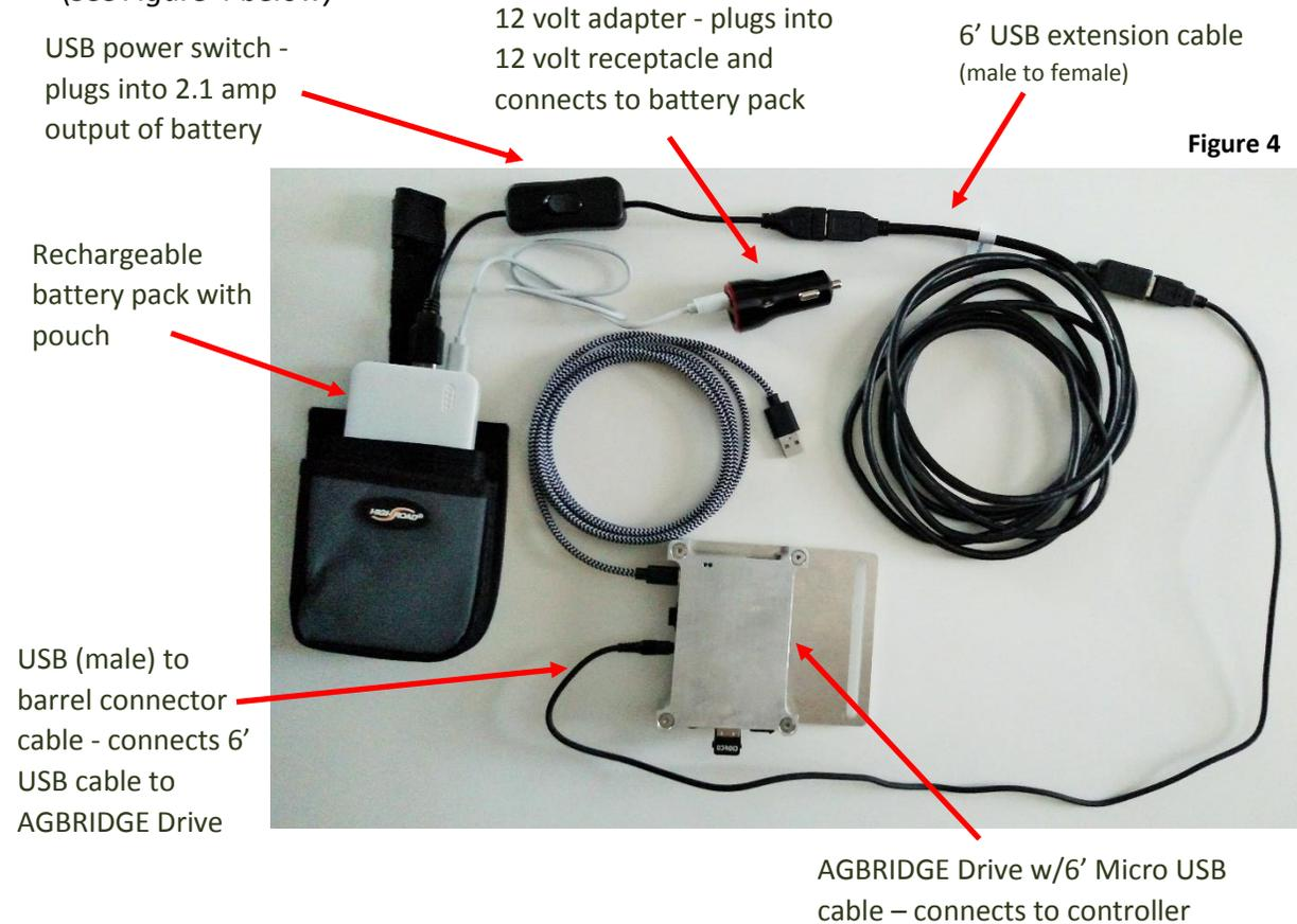
**Section 3 Note 1:** The rechargeable battery pack charges and discharges simultaneously when connected to a powered 12V receptacle. It is preferable to use a 12V receptacle that is connected to “switched power” if possible; however the current draw when charging is typically not enough to cause significant power drain of the equipment’s battery system. **Always be sure to toggle the USB power switch to the “off” position when finished.**
